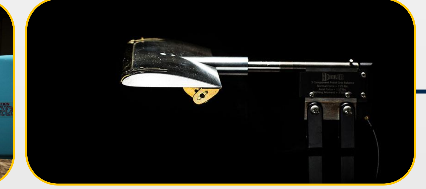
Figure 5 - Clark Y-14 on 3-Force Probe
